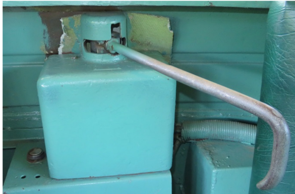
Brake & Shift Handle Insertion/ Removal Position “b”
