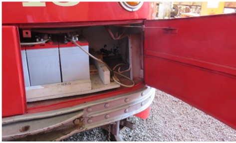
Battery Compartment with Right Door Open
