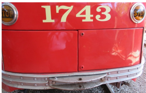
Battery Compartment On Rear of Streetcar
